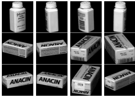
Figure 10. Prototype views selected for two different 3D objects from the COIL dataset using the algorithm described in Section 5.2. With this approach, views are allocated adaptively depending on the visual complexity of an object with respect to viewing angle.
